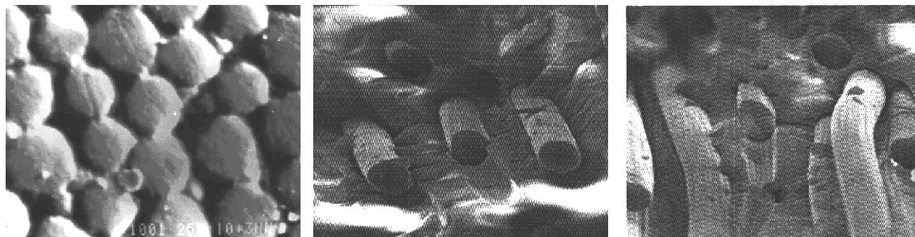
Fig. 4. Microstructure of the Steklarm composite.
